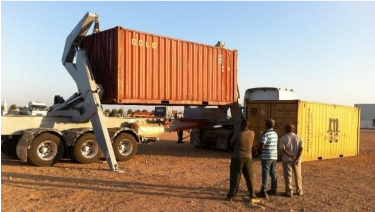
Product Name: SB450RSH2040 A 20/40 foot Semitrailer Sidelifter. Cranes sliding on long triaxle semitrailer.
